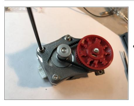
Rotate motor on its pivot bolt to take up belt slack. You don't need to make belt super taught like the X
